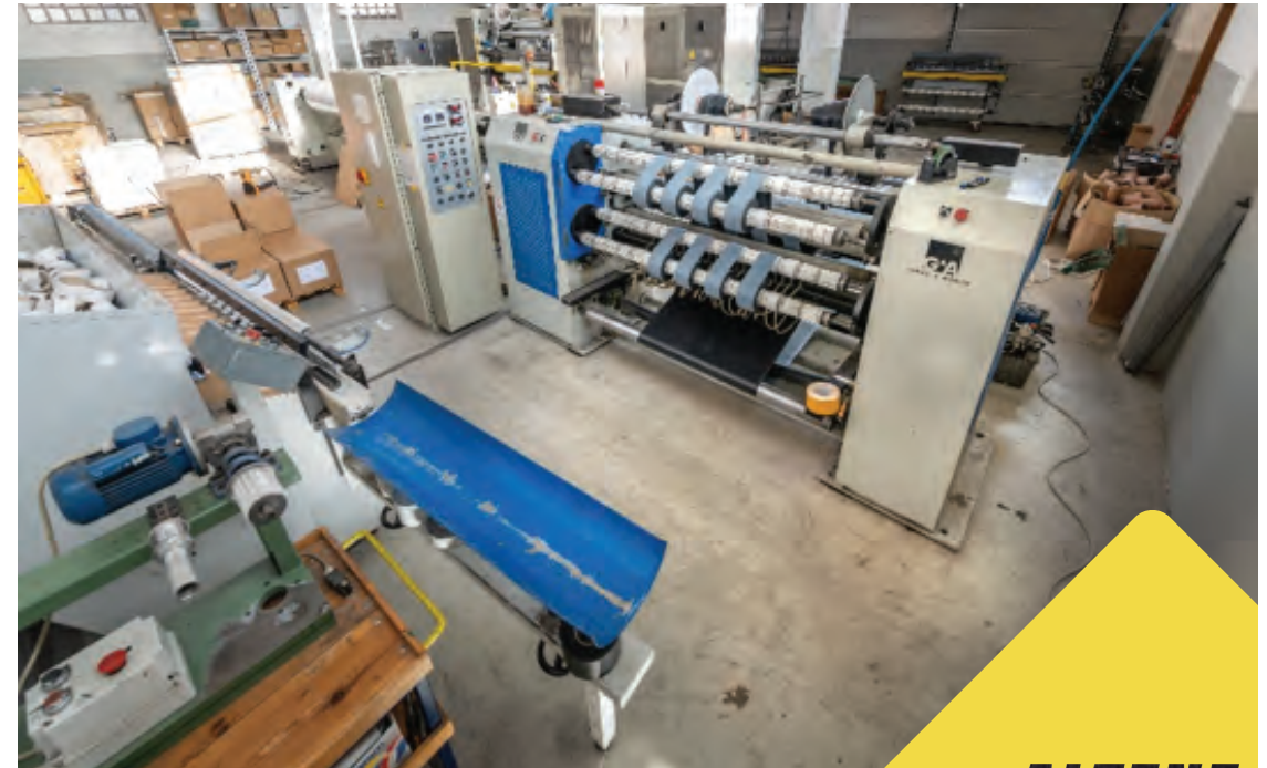
Cutter size 200, small and versatile. Possibility of winding the tape on 41 and 76 Subbi.
