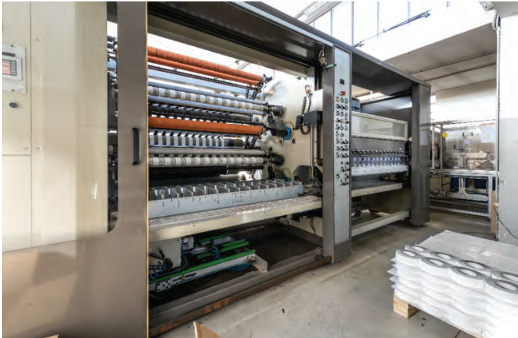
All-automatic cutter size 400, from loading master rolls to unloading rolls ready for packing
