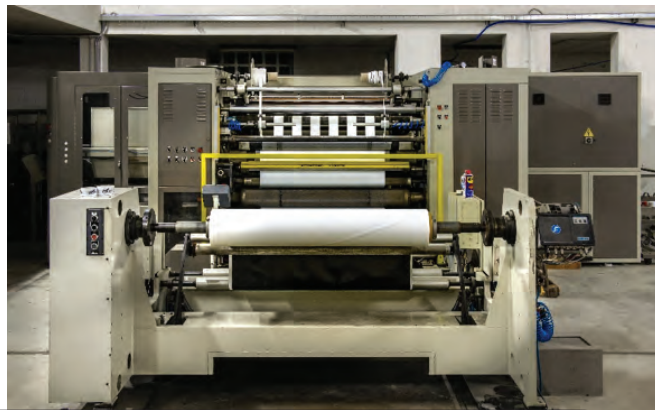
All-automatic cutter size 400, from loading master rolls to unloading rolls ready for packing
