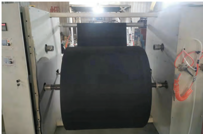
Production of master rolls of various thicknesses ready for the cutting line.
