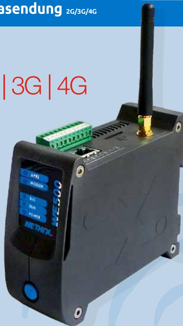
**We500** is a complete, flexible, and high performance platform that provides wireless unattended remote monitoring and control with 2G, 3G or 4G connectivity.
