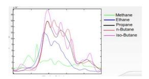
ETG 6700 provides selective measurements of the hydrocarbon species and carbon-dioxide, and calculates the calorific value, Wobbe Index and other gas properties in real time.
