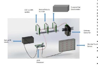
The ETG 6700 it's composed mainly by the Tunable Filter Spectrometer which's capable of high-accuracy fuel gas composition measurements every 5 seconds. The ETG 6700 Gas Analyzer provides selective measurements of the hydrocarbon species and carbon-dioxide, and calculates the calorific value, Wobbe Index and other gas properties in real time. The analyzer provides real-time data through Modbus digital interfaces. Other components are:
