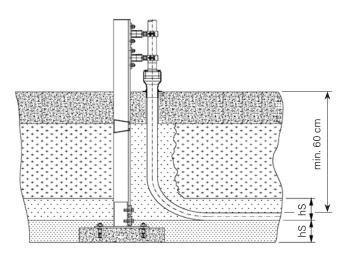
Thickness of the sand bedding hS = 10 – 15 cm, grain size < 2 mm
